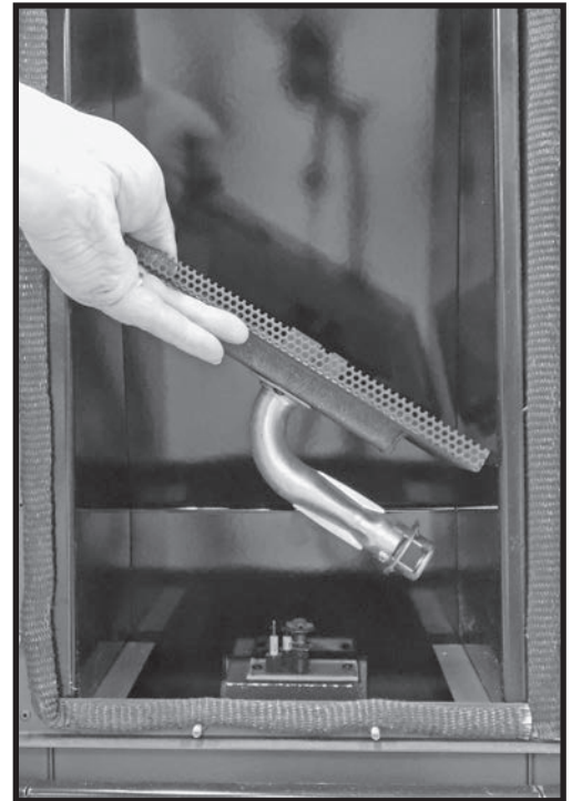
Figure 26: Burner tray insertion and removal.
