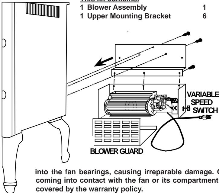
Your EP62-1 blower kit comes complete with a variable speed switch that is used to turn the blower on and off as well as adjusting the blower speed.
