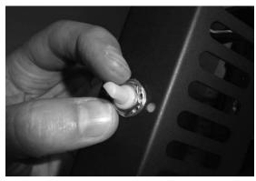
4 Connect the two wires from the Rheostat to the black wires in the control housing. Install the blower control knob and return the assembly to its original configuration.
