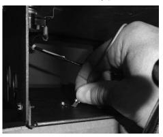
9 Connect the two remaining connectors on the blower assembly harness to the two wires marked "rheostat" that come down from the control box. Insert the two included plastic wire restraints into holes in the floor of the valve area and clip excess wire in place. Make sure no wire will make contact with hot surfaces.
