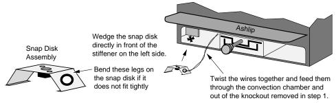
2A Secure the snap disk wires in place following the directions below. Go to step 3.
