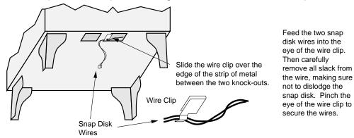
NOTE: The wires must be properly secured to prevent them from contacting the firebox and shorting out the blower circuit.
