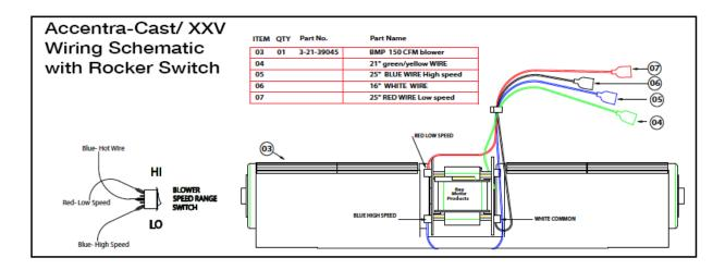
XXV/ Accentra-Cast units made without a rocker switch will ONLY have wires connecting for the Dark Blue and White. The spade on the motor for the red wire MUST be capped to prevent an accidental shorting of the circuit. Connecting a blank female wire terminal is the easiest way to do this.
