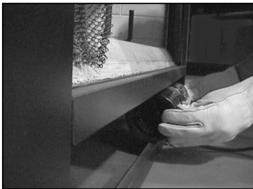
Figure 5 - Rotating the Fan into Position
