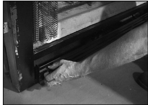
Figure 1 - Removing the Lower Grille
