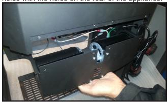
5. Secure the fan by fastening x6 screws to the appliance (note: x2 screws fasten into the firebox bottom).
