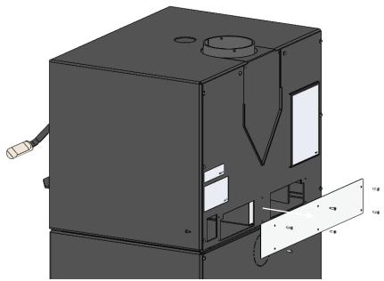
2. With outer fan cage uninstalled and fan kit aligned with slots in rear of unit, position rheostat into outer left slot and install into hole on left side of firebox can with supplied rheostat nut.
